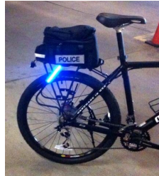
SIDE LIGHTING All RED or All BLUE Red operates in non-Code-3 and Code-3 Blue operates in Code-3 ONLY
